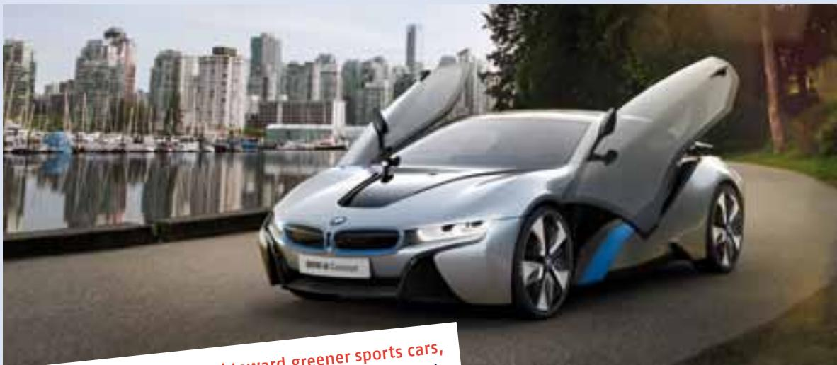
Representing the trend toward greener sports cars, the plug-in **BMW i8 concept** combines an electric drivetrain with a three-cylinder combustion engine. This hybrid configuration ensures that the roadster only consumes as much fuel as a small car.
